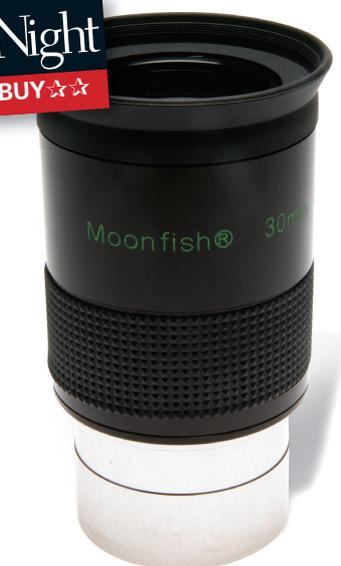
that the field stop is just under 41mm in diameter. Our tests revealed that figure to be 44.8mm, delivering a staggering 4.3° field with the Tele Vue-85 refractor. The view was coma-free out to 70-75 per cent of the field radius with good contrast and colour correction.
